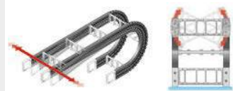
3D movements: the driver connection can be moved laterally and can be rotated by up to ± 30°
