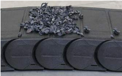
Example: Cover system with chips
