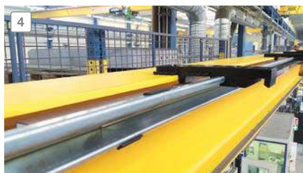
Hanging and orienting the guidance trough and assembly of the holder clamps
